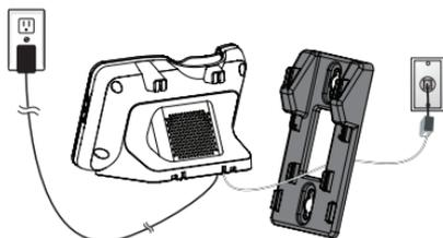
3. Position the lower portion grooves on the telephone base to the lower portion tabs (marked **B**) on the wall mount bracket. Make sure the upper portion grooves of the telephone base are above the upper portion tabs (marked **A**) on the wall mount bracket. Push the telephone base down until it clicks securely in place.
