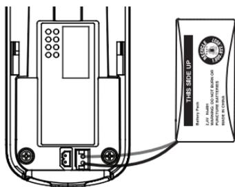
2. Place the battery with the label **THIS SIDE UP** facing up and the wires inside the battery compartment.
